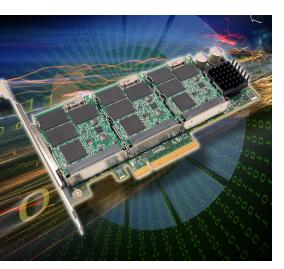
The LSI WarpDrive SLP-300 enables very high IOPS to accelerate high demand applications like real time network analysis and SEIM. Where standard hard drive technology might not be able to keep up, the WarpDrive card offers a PCIe plug-in solution that easily installs into existing server platforms without taking away precious system resources from the CPU or memory.
